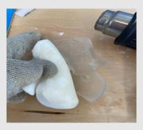
3 Stretch the heated piece of Erkoflex to the same thickness of the pad and adhere it to the pad
