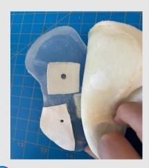
Using dacron or tape, reinforce the area where you are going to place the rivets. With a hole punch, punch a hole that is slightly smaller than the rivet post
