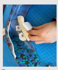
Rivet the pad to the device and glue thermofoam pad over
